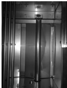
Straight Burner (Standard) located underneath the briquette trays.
