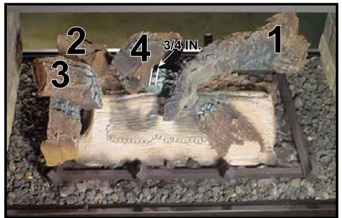
STEP 5. LOG #4 (SRV2005-703): Locate the sharp notch on log #4 against the grate tine as shown. The smooth cutout on the bottom of log #4 should rest on the burner surface. The side of Log #4 must be 3/4 inch from the nearest port hole on the right side of log #4. **DO NOT** cover any port holes.
