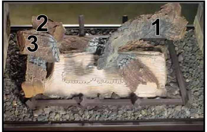
STEP 4. LOG #3 (SRV2005-702): Position log #3 as shown by leaning it against log #2 and resting the other end on the peak of the burner. **DO NOT** cover any port holes.
