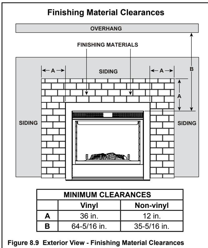
Figure 8.9 Exterior View - Finishing Material Clearances
