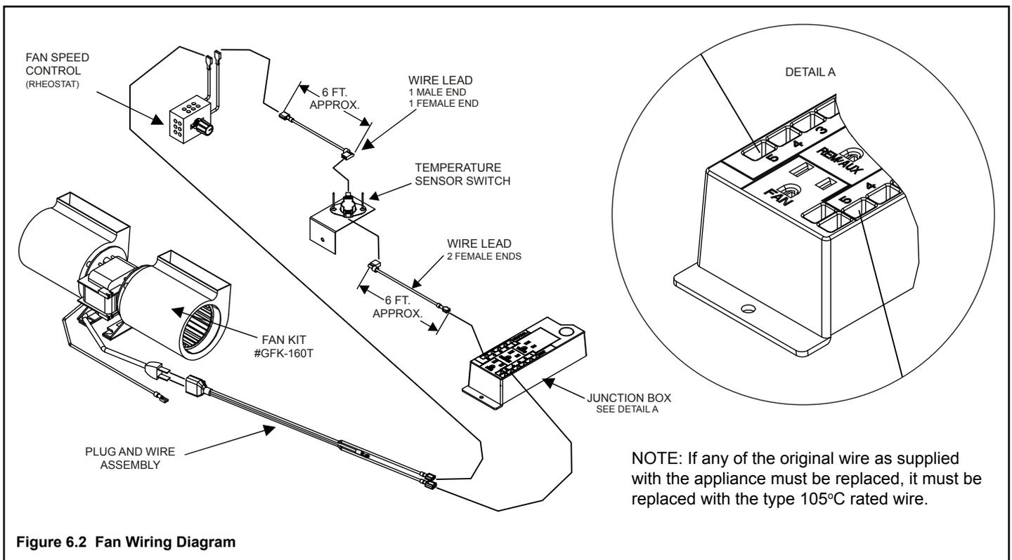
**NOTE:** If any of the original wire as supplied with the appliance must be replaced, it must be replaced with the type 105°C rated wire.
