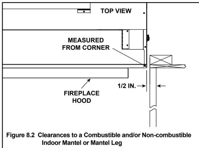
Figure 8.2 Clearances to a Combustible and/or Non-combustible Indoor Mantel or Mantel Leg
