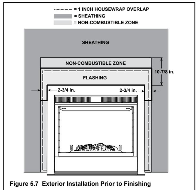
Figure 5.7 Exterior Installation Prior to Finishing
