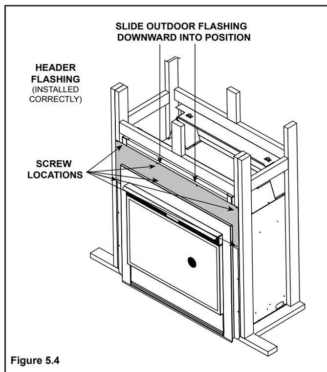
Seal flashing to exterior of building using high temperature silicone sealant. Attach to building using holes provided on the top of the left and right sides of outdoor flashing. See Figure 5.4.
