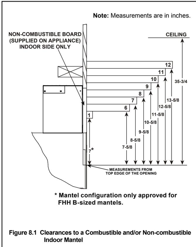
Figure 8.1 Clearances to a Combustible and/or Non-combustible Indoor Mantel
