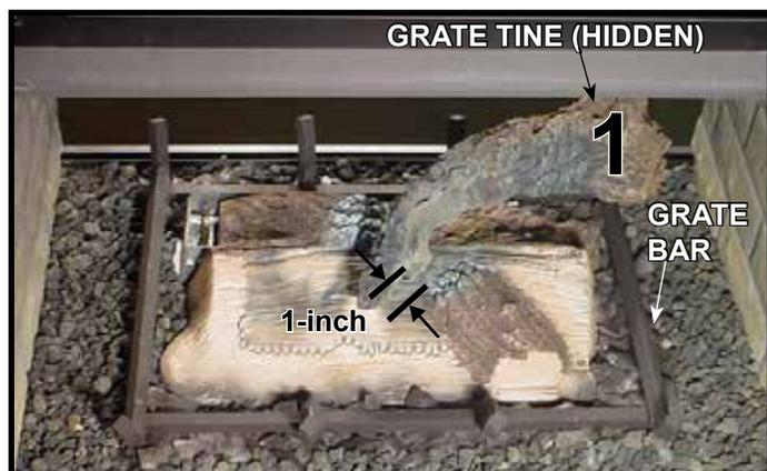
**STEP 2. LOG #1 (SRV2005-701):** Use the indent on the bottom side of the log to position the large end of the log onto the grate bar as shown. Slide the log back until the indent engages the grate tine as shown above. Position the thin end of log #1 one inch from port pattern as shown.
