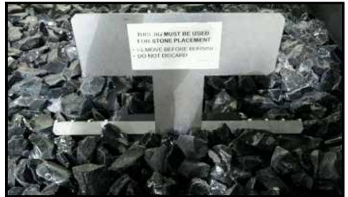
Figure 9.7 Rock Placement Jig
