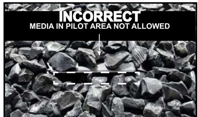
Figure 9.9 INCORRECT Media Placement
