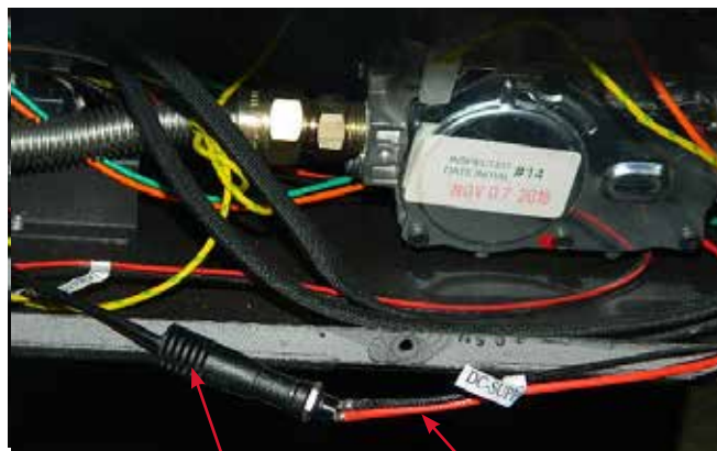
DC supply wire from wiring harness
